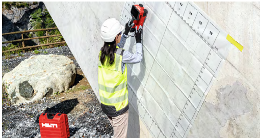
a) Scanning for ferrous objects
