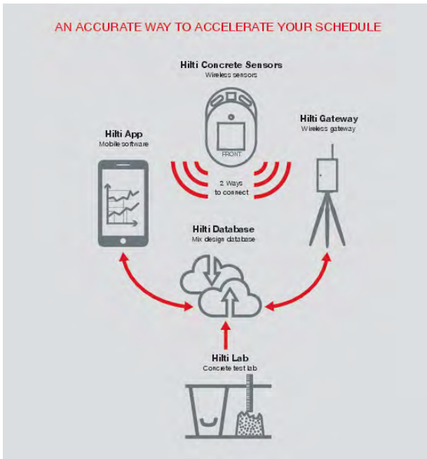
Fig. 9.21: Hilti concrete sensor system solution
